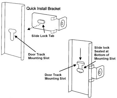
Step 12: Install <u>Wireless</u> Infrared Safety Sensors Wall Mounting Bracket
